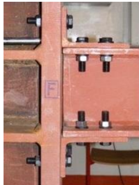
Rys: Behaviour of stiffened flange cleat joints, D. Skejic, D. Dujmovic, D. Beg
