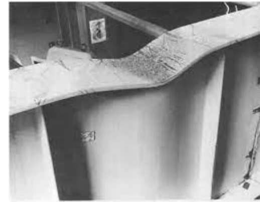
Rys: Web Buckling of High Strength Steel Plate Girders Induced by Bending Curvature, S. Nascimento, J. Pedro, A. Biscaya, Wiley Online Library, 9 III 2020
