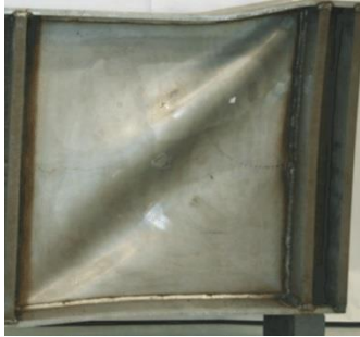
Rys: Saliba, N. Gardner, L. Experimental study of the shear response of lean duplex stainless steel plate girders. Engineering Structures. 1 / 2013
