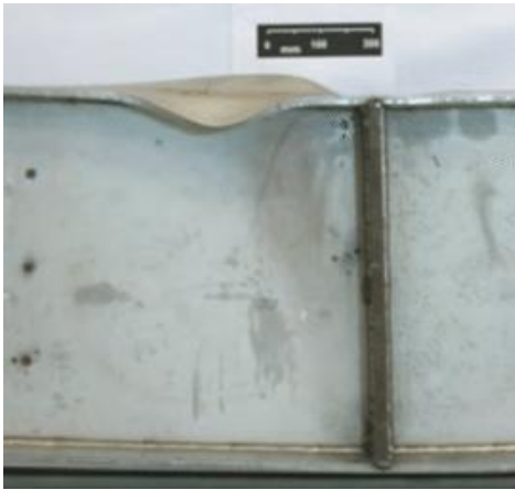
Rys: Saliba, N. Gardner, L. Experimental study of the shear response of lean duplex stainless steel plate girders. Engineering Structures. 1 / 2013
