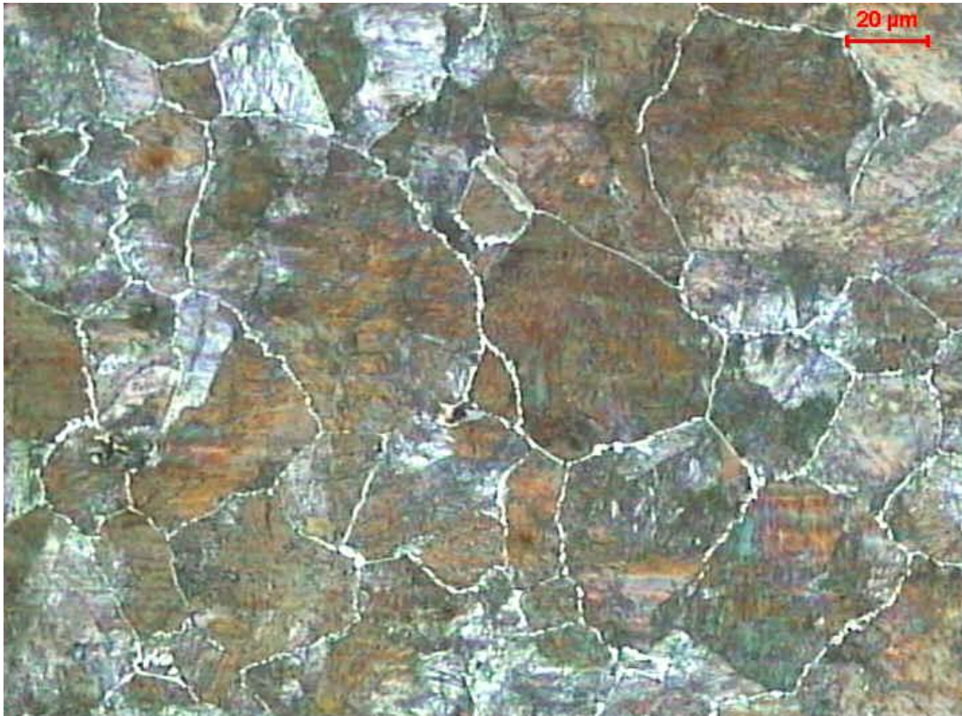
Perlite + little quantity of ferrite (steel)
