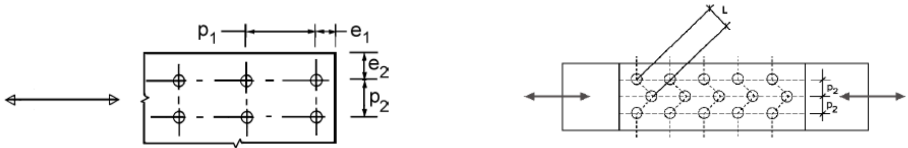
Distances according to EN 1993-1-8 fig. 3.1
